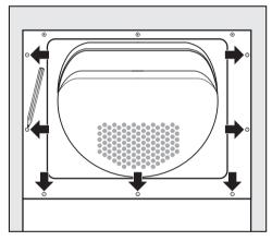
Mark the fixing points on the back of the front panel through the holes in the machine door plate (see arrows in the illustration).
